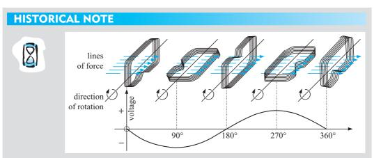
In 1831 **Michael Faraday** discovered that an electric current was generated by rotating a coil of wire in a magnetic field. The electric current produced showed a voltage which varied between positive and negative values as the coil rotated through  $360^{\circ}$ .
